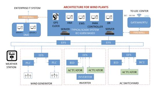
Architecture layouts for RE plants (with ON-Premise SCADA) are as under:
